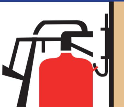
Fire extinguishers should be securely hung on wall brackets.
